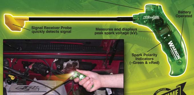
The kV/Arc Quick Probe is easy to use — simply place the probe over the ignition wire. Each time the unit detects a spark firing, it will flash the Super Bright LED strobe indicating a spark-firing event with sufficient arc duration. Then press the button and the unit measures and displays peak kV on the LCD display.
